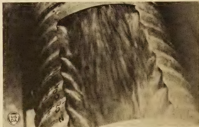
FIG. 10.—Water flowing in 24-inch corrugated metal pipe. Depth of flow 1.82 feet, discharge 17.88 second-feet. Note disturbance of filaments of flow due to corrugations.
